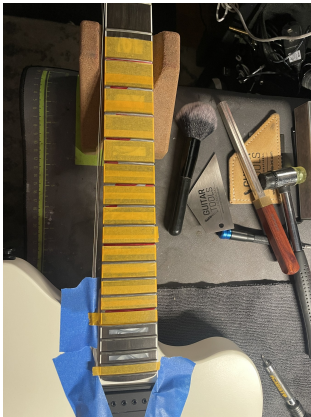
Masked fingerboard before/while performing fretwork.
