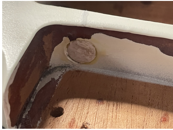
Maple plug installed in pocket area.
