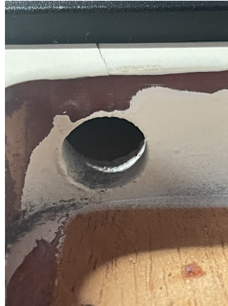
Close-up of routed pocket passage and crack area before repair.
