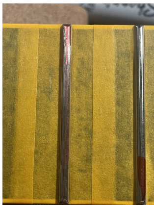
Close-up of polished/corrected fret area.
