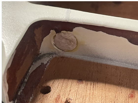
Maple plug installed and glued into the compromised pocket area.
