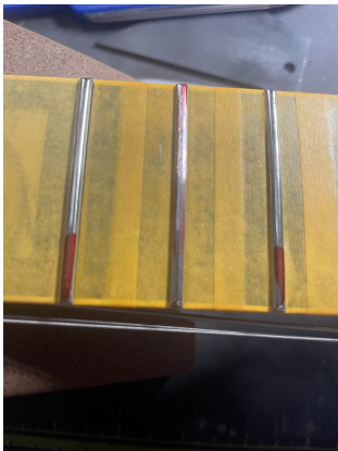
Spot leveling/crowning/polishing documentation.
