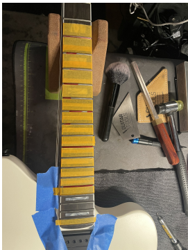
Fingerboard masked for fret work.
