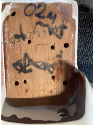
Neck removed; neck pocket exposed for structural inspection.
