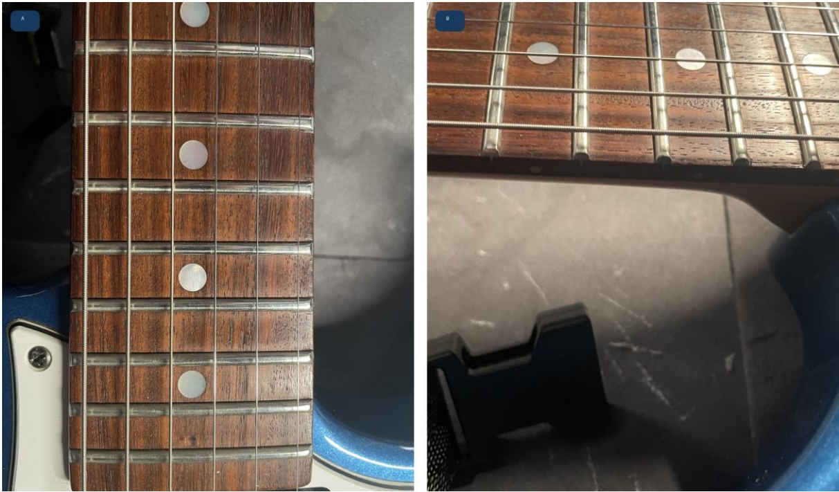
Figure 2. Incoming fret condition. (A) Broad view of the rosewood fingerboard and original frets. (B) Detail view showing flattened crown surfaces and localized playing wear. Source: Service photograph supplied with work order.
