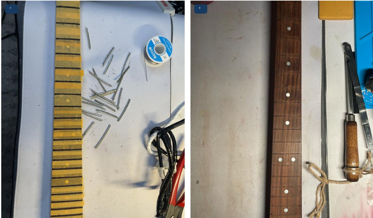
Figure 4. Fingerboard after extraction. (A) Removed fretwire beside the protected board. (B) Cleaned slot field with the original compound-radius rosewood surface exposed. Source: Service photograph supplied with work order.
