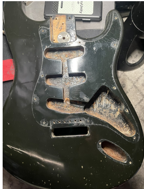
Old shielding and adhesive/residue after removal; corrosion/salt contamination was documented and cleaned.
