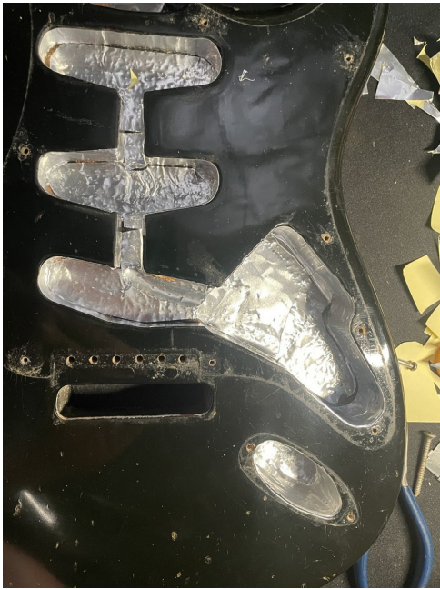
Shielding work after cleaning and re-shielding the cavities.
