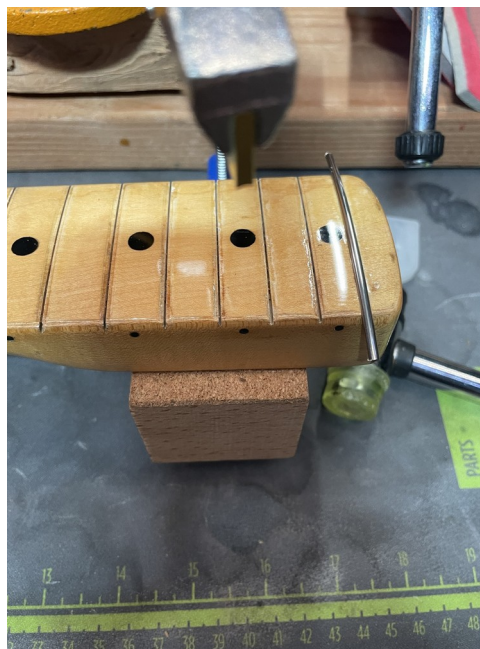
New frets seated into the corrected maple board.
