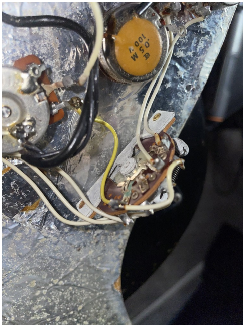
Potentiometers, wiring, and control cavity condition documented during electronics inspection.
