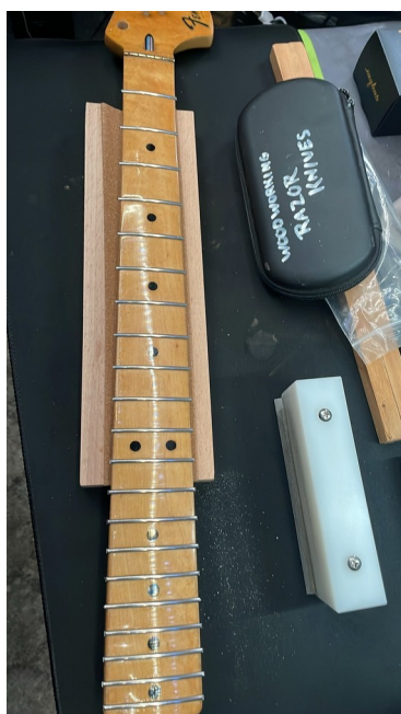
Fret installation complete across the board before final end work and leveling.
