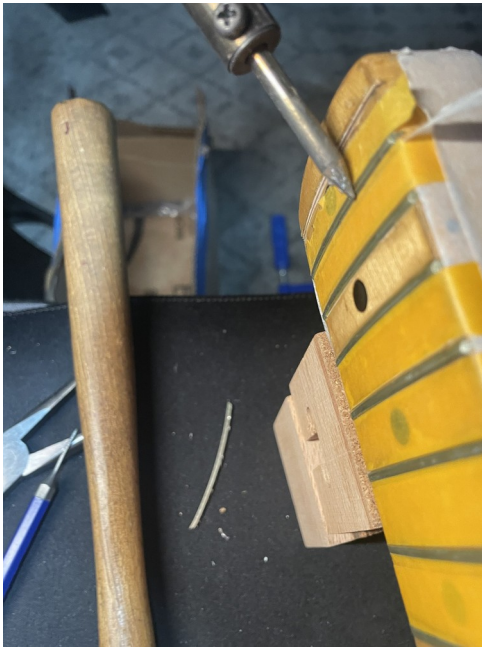
Controlled fret extraction began with localized heat and support to protect the aged finish.
