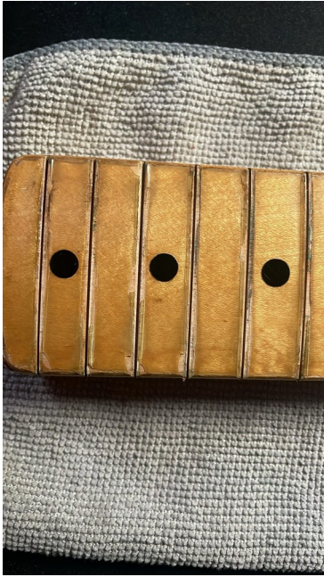
Fret slots and board surface after removal, before final finish/slot preparation.
