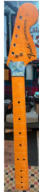
Color-matched finish work on the maple neck after sanding and tint adjustment.
