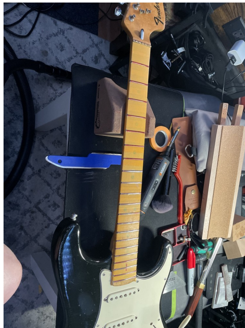
Refret level/crown/polish work in progress after installation.
