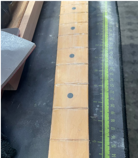
Progressive sanding across the board to remove humps and prepare for a playable refret.
