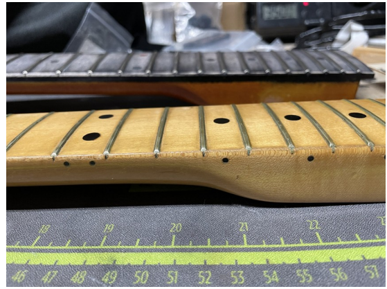
Upper-board condition before fret removal and board correction.
