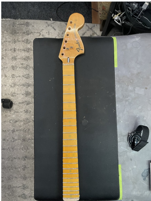
Fret ends trimmed and dressed after pressing.
