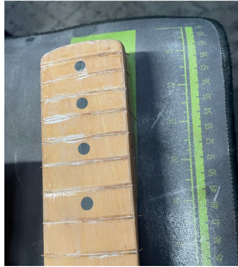
Poly/finish leveling and board correction after fret removal.
